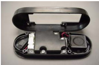
UIB - USER INTERFACE Retainer & Assembly
