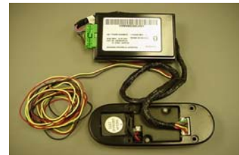
WIRE HARNESS Main Harness – UIB to HFM with power leads
